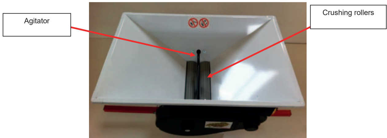
Fig. 1 Main parts of the GRAPE CRUSHER
